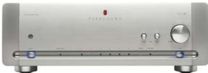
Parasound's Halo JC 2 is a remote-controlled, solid-state preamplifier with switchable absolute polarity, a rear-panel IR repeater input and loop out jacks, four 12-V trigger output jacks, and a two-way RS-232 serial port.
